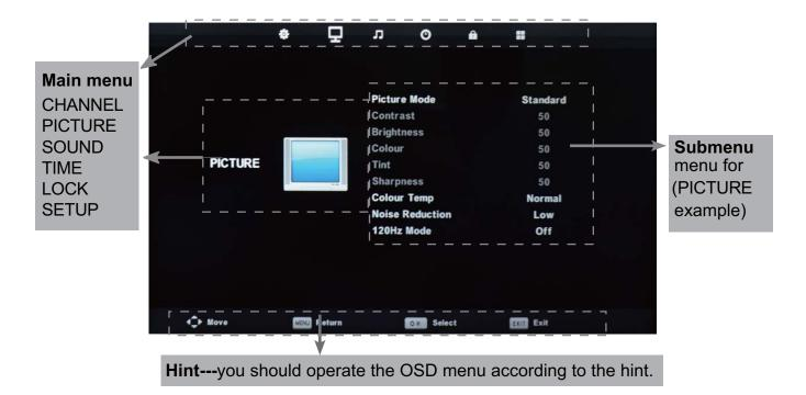
Use </> button to select the main menu, and press  $\lor$  button to enter the submenu. In the submenu, use  $\land/\lor$  button to select the function item, press </> button to adjust/setup, or press **OK** button to enter the submenu.
