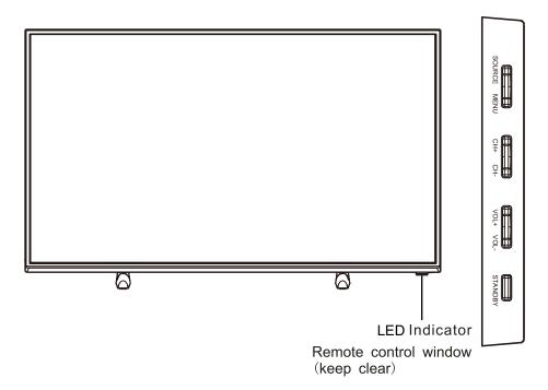
1). (IR) Infrared Receiver: Receives IR signals from the remote control. (Power on/Standby)LED Indicator: Press 4/1 (POWER) to turn on and off.
